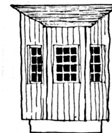
NO "MODERNIZED" BAY WINDOW WITH VERTICAL SIDING
